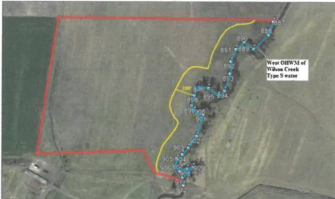
Above: Gps mapping of the west ordinary high water mark of Wilson Creek, a Type S water. The 100' buffer is also depicted in yellow.
